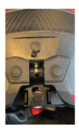
3. Lubricate the lever with 1 drop of chain lube in each cavity of the lever. Do not use excessive amount of oil. 1 drop is enough.
