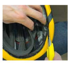
3. Remove the Occigrip. Loosen the velcro on the Mips Air LFL. You do not need to remove the Mips Air LFL from the helmet, ONLY loosen it from the Occigrip.
