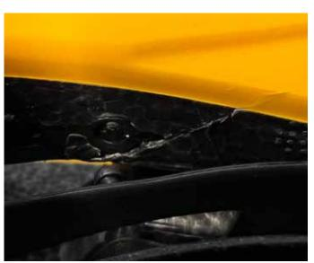
5. Position the occigrip hanger and place the part in the correct place. Tighten the screw so that the Occigrip hanger has some resistance when moving up and down.
